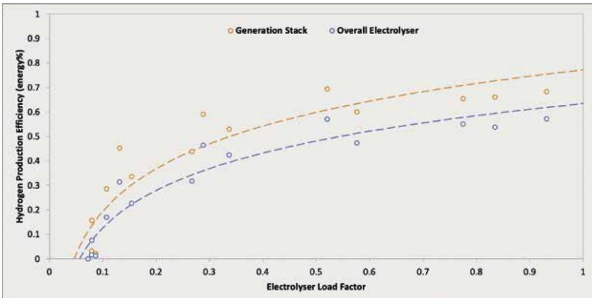
Figure 18: Electrolyser operational efficiency
