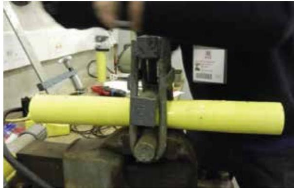
**Figure 4: Squeeze off demonstration**
