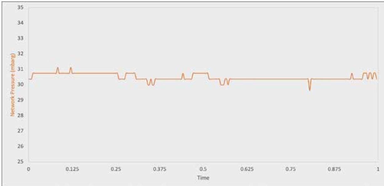
**Figure 20: Typical network pressures**
