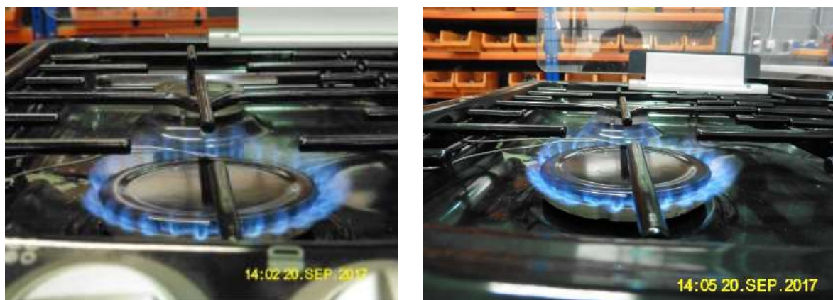
Figure 2: Cooker hob flames (LHS – Methane, RHS – 28.4 vol% Hydrogen)
