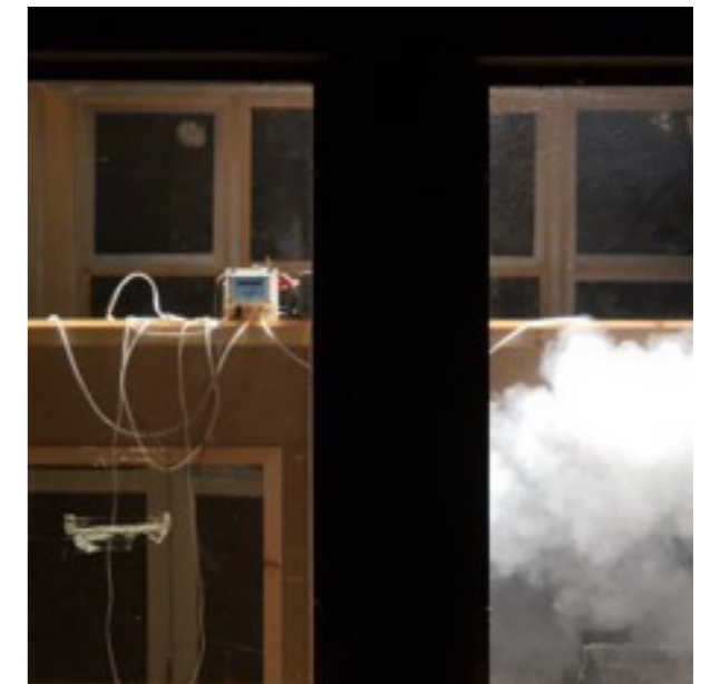
Figure 4: Experimental setup showing how hydrogen blended gas accumulation characteristics were tested.
