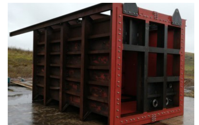
Figure 5: Image of bespoke container developed to run hydrogen blended gas explosion characteristic experiments.
