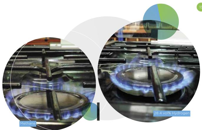
The gas boiler testing focused on flue gas analysis alongside internal temperature measurements and flame ionization currents. The flame characteristics for each test gas, including up to 28.4 mol% hydrogen, were stable with complete combustion being achieved. As expected, the carbon dioxide readings reduced by up to 0.5 mol% with the addition of hydrogen.
