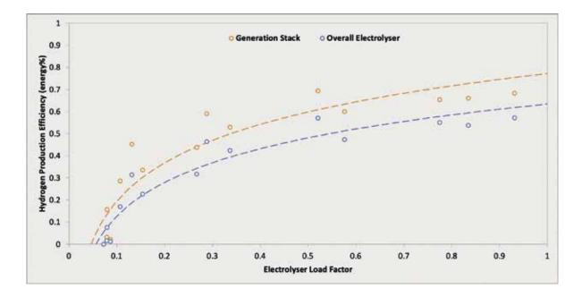
Figure 18: Electrolyser operational efficiency
