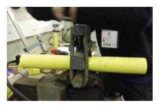
Figure 4: Squeeze off demonstration
